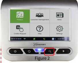
After the chip is successfully scanned, you can enter into the final operation interface. Click to switch functions "RESET", "CHECH" and "SCAN", and press the "Confirm" button on the JIG or Unismart device to carry out the chip operation.
